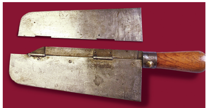
Luther tool broken during Fort Snelling trials.
